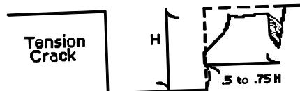
**SLIDING** (or sloughing) may occur as a result of tension cracks, as illustrated below.
